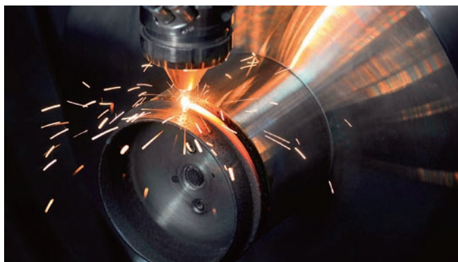
► EQUIPMENT MACHINING: In DMG's hybrid machine, the laser ensures the deposition of the material. 64
