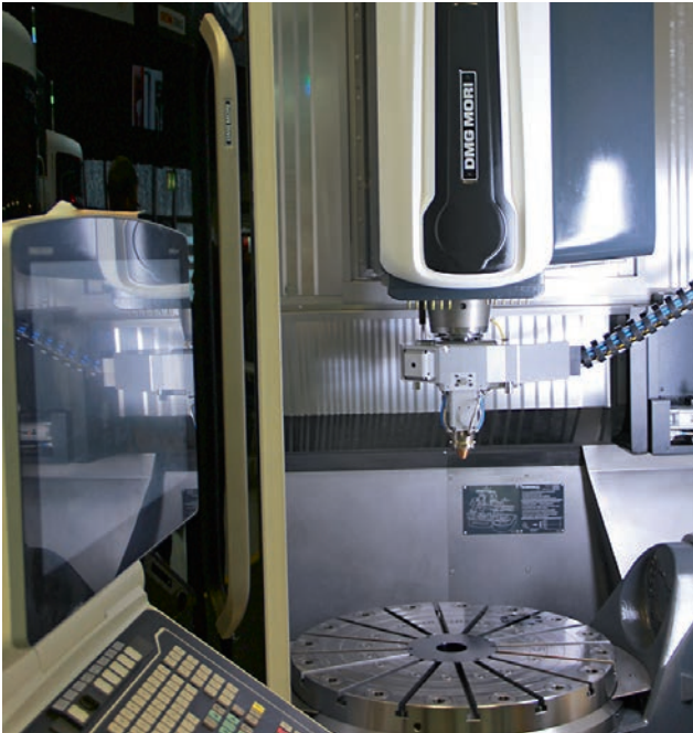
View of the work area of the DMG Mori 65 3D hybrid machine. The laser head can be changed automatically.
