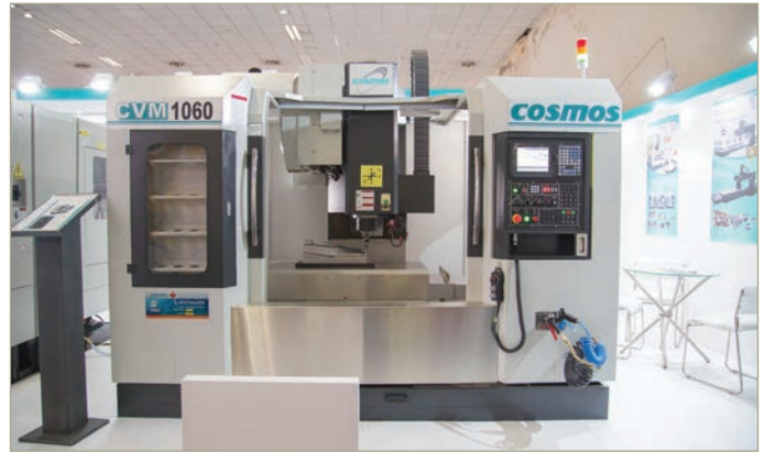
Mitsubishi's controller has been installed in COSMOS' CVM 1060
