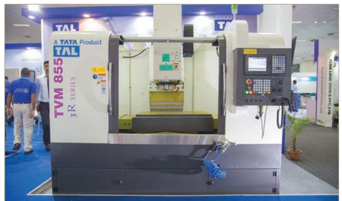
TAL's TVM 855 machine with Mitsubishi's controller
