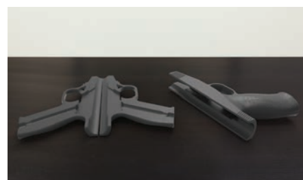
CNC machined pistols have to be created in two halves and then joined together to complete the part.
