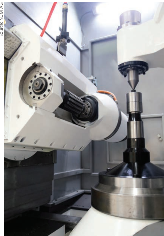
The Betek six-axis YK3132Z gear hobber accommodates gear blanks up to 320 mm in diameter.
