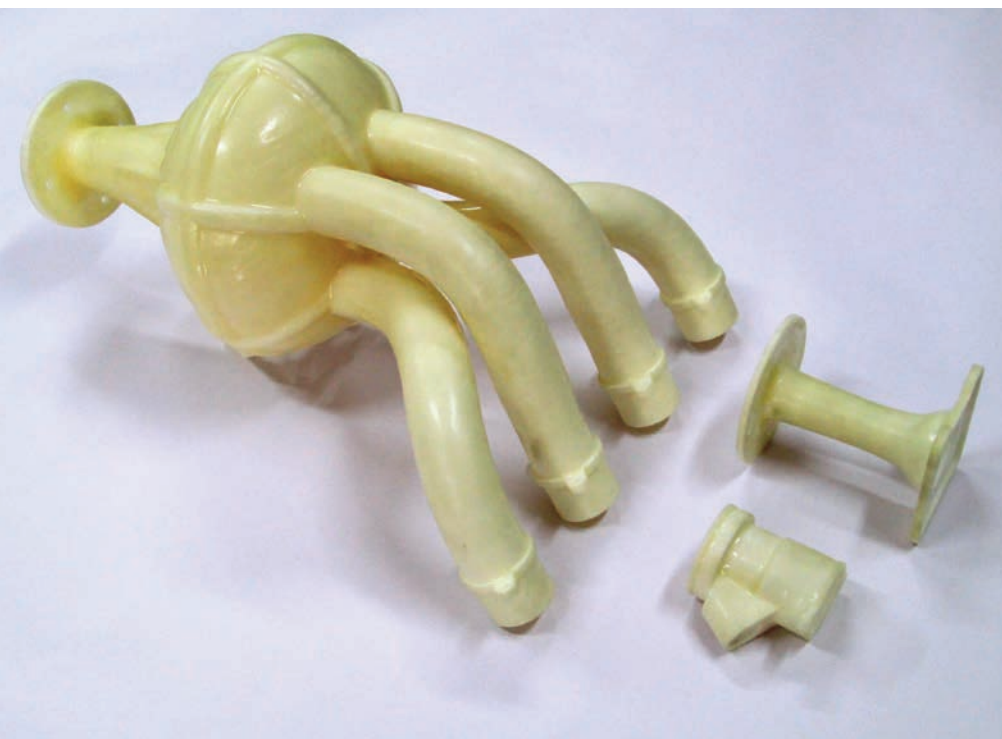
3D printed model of an air intake system used in formula cars.
