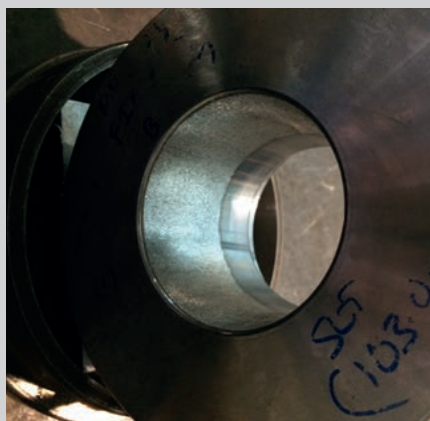
Scratch and serrations-prone inner diameter of a forging die that was coated. Carbide coating is seen as silvery coarse layer.
