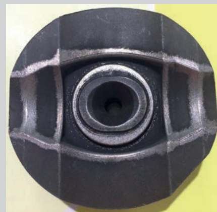
Sensitive areas of the die were protected with carbide coating. It is seen as silvery layer on edges of die profile.
