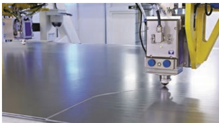
As the Schuler line uses fiber lasers, no dies are required – in contrast to conventional blanking lines.
