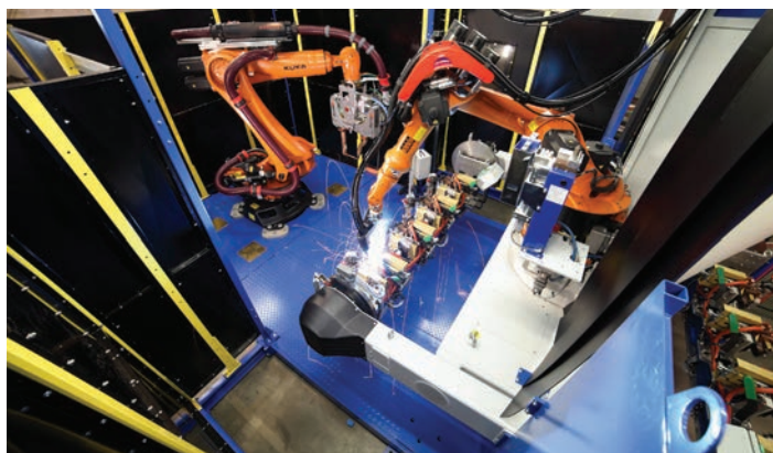
► WELDING: The streamlined design of the wrist ensures that the robot enjoys minimal disruptive contours and maximum freedom of motion.
