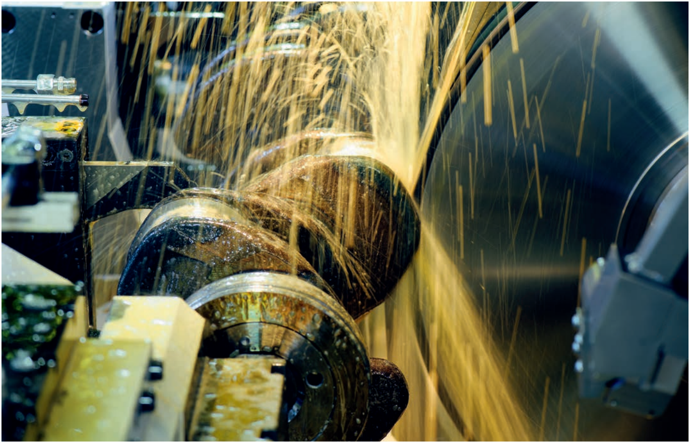
The largest JUNKER platform built to date will soon be put to use for the grinding of crankshafts.
