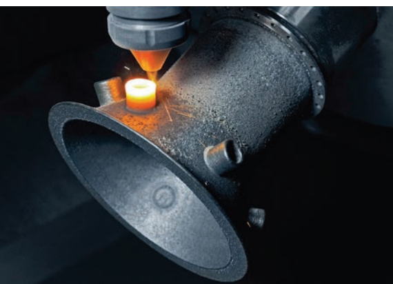
► ADDITIVE MANUFACTURING: The hybrid machine allows milling and additive manufacturing in one fixture.
