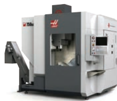
The UMC-750SS is a five-axis, 40-taper model that offers travels of 762 x 508 x 508 mm, 30.5 m/min rapids and an integrated high speed, dual-axis trunnion table.
