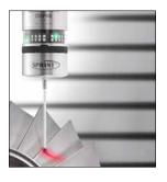
Renishaw has launched Sprint, a highspeed analogue contact scanning system for CNC machine tools. This system incorporates a new generation technology that delivers a step-change in the benefits of process control. It enables fast and accurate form and profile data capture from both prismatic and complex 3D components. For blade manufacture,
