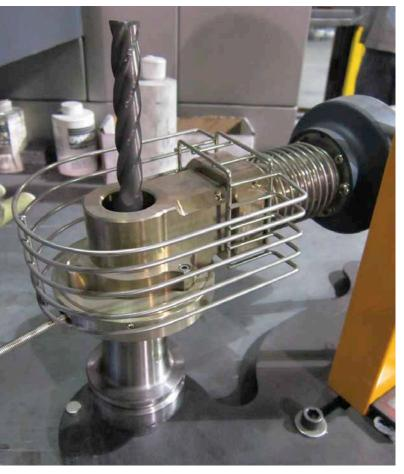
► HIGH SPEED MACHINING: The shrink-fit tooling offers the runout and rigidity required for effective high speed machining of mold blocks as hard as 60 HRc
