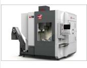
The UMC-750, universal machining center from Haas Automation, offers travels of 762 x 508 x 508 mm and an integrated dual-axis trunnion table. This machine is equipped with an inline direct-drive, lowheat 40-taper spindle (8100 rpm
