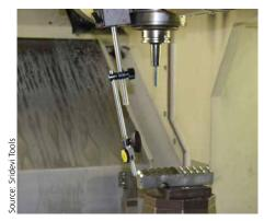
Inspection being conducted on the contoured shape of completed job at Sridevi Tools
