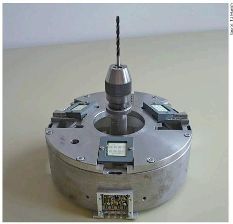
FIG 2: This clamping system with mounted radar sensors recognizes the crash danger and stops the drives before the collision
