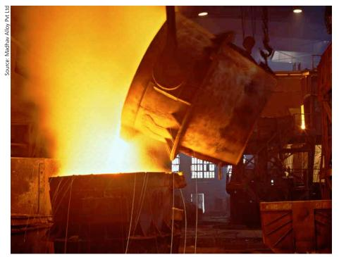
Typical casting of molten iron at a steel plant
