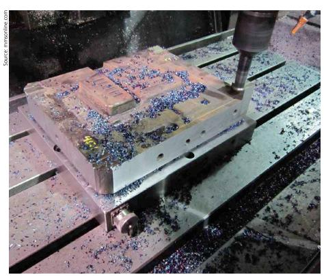
Electropermanent magnetic chucks on the company's sinker EDMs and machining centers speed setups and enable multiple jobs to be fixtured at once
