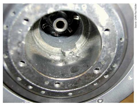
FIG 1: The damaged interior of a machine spindle after a collision of the tool with the workpiece
