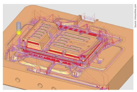
The CimatronE CAM software precisely calculates the stock remaining after each tool path and uses that information to optimize subsequent cutter moves. This has virtually eliminated gouging, which was common with the company's previous CAM package.
