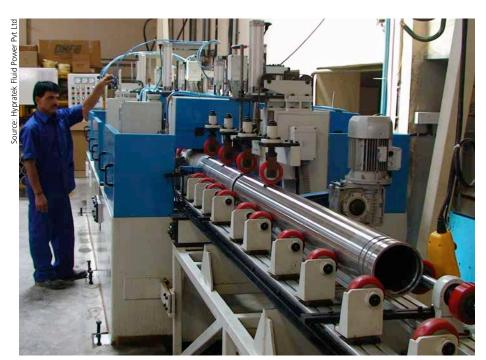
The machine is user-friendly and easy to set up; thereby, requiring only single worker to monitor the grinder process
