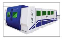
coated and textured metal sheets. It can cut a 20 mm of steel with a 3 kW fiber laser with high quality standards. It further offers butter cut, striation free edges at thicker metals, less angular distortion and enhanced cutting through well monitored and controlled pressure of the assist gases. Moreover the machine also features bevel and tube cutting options.
