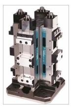
Fresmak Arnold Precision Engineering's twin high pressure vice allows to clamp the different types of components at much ease and less cost. This comes with a spindle integrated with a hydraulic pressure booster, which boost the pressure up to 40KN just by using hand rotational movement. It has a pressure regulator that controls the clamping force at different intervals. Thus it enables clamping rigid components at high pressure and slender components at accurate and lighter pressures.
