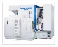
significant reductions in cost per piece, when compared with the gear shaping process, for example. The tool concept gives the Power Skiving process unprecedented flexibility and simplicity of process management. This makes the process for gear diameters up to 700 mm, swing diameters up to 850 mm and modules up to 8 mm equally suitable for small lot production runs as well as mass production.
