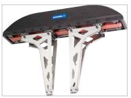
gripping force of 2,500 N and a variable stroke per gripper finger of up to 160 mm. The decoupled re-circulating ball carriages ensure that the acting moments will be optimally distributed onto the whole rolling elements.
