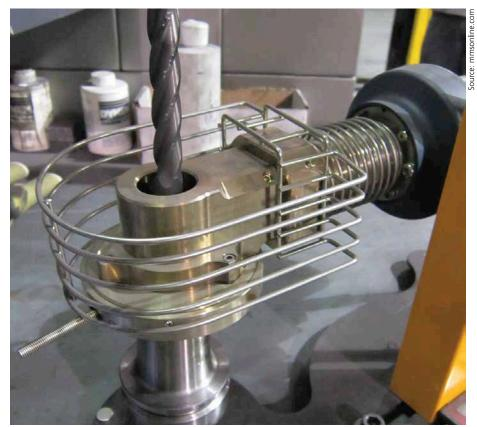
The shrink-fit tooling offers the runout and rigidity required for effective high speed machining of mold blocks as hard as 60 HRc
