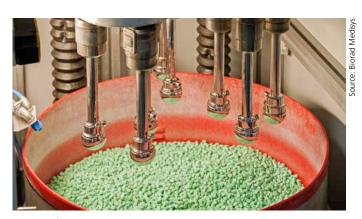
Cast or forged implants go through processes like three-stage OTEC dry polishing
