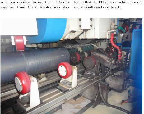
The job passing to the multihead belt grinding machine at the Hypratek facility
