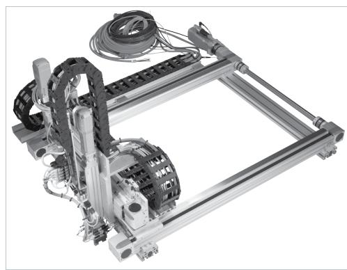
► MOTION CONTROL: A three-dimensional gantry consisting of horizontal gantry axes and a vertical drive, that can be used universally for light to heavy workpieces
