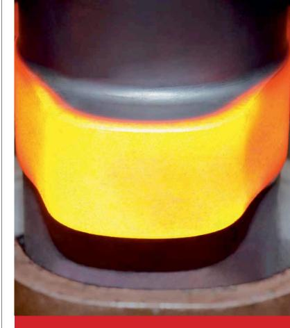
Induction can heat a cam lobe to 950°C in five seconds.
