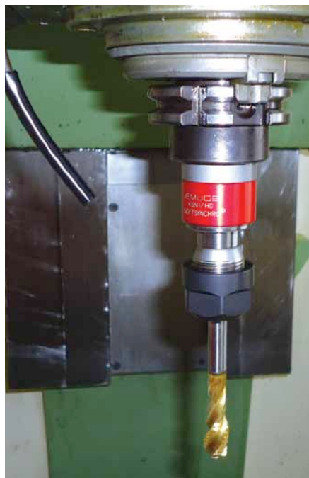
Tap holders provided by Emuge to Bosch Chassis Systems led to an improvement of more than 15 per cent and eliminated problems such as thread damage and leakage
