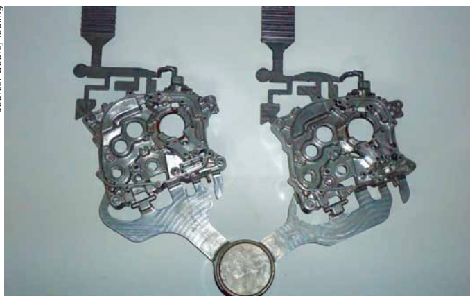
Godrej Tooling has innovatively developed twin cavity crank case dies that can run in the same machine as single cavity die
