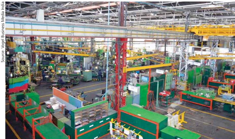
The shopfloor of Godrej's tooling division is lined with medium to large high speed CNC milling machines and very large double column milling machines
