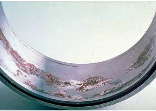
Fretting corrosion in the bore of an inner ring
