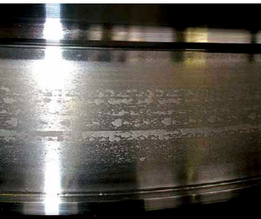
Typical surface distress/microspalling in wind gearboxes
