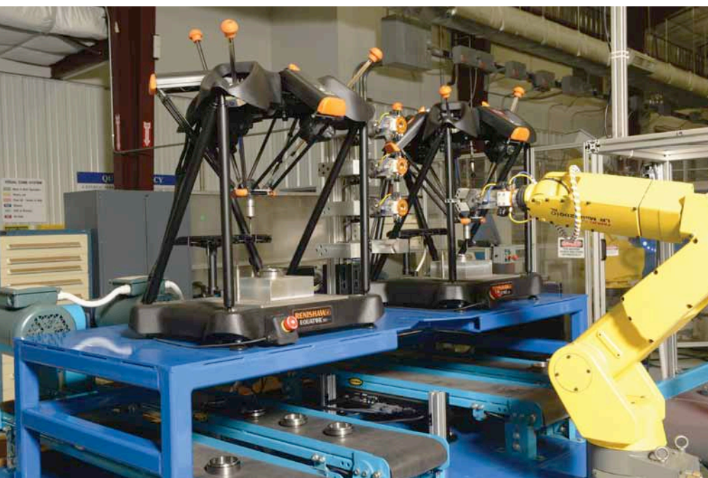
In development - Conroe's new dual Equator automated cell
