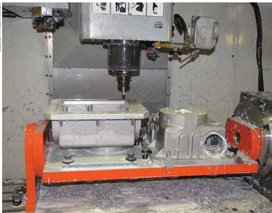
Using trunnions and quick-change plates with Jergens ball locks in place of old homemade fixtures helped Indelac reduce cycle time by 40 per cent
