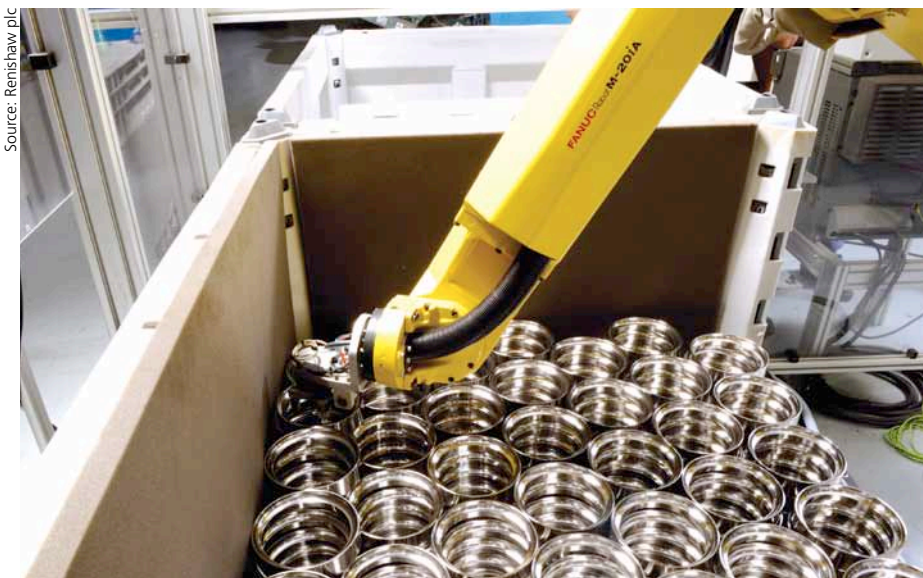
An automated FANUC robot boxes and palletizes parts
