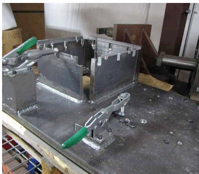
Indelac's old fixtures included manual clamps, angle plates and plugs. With this workholding methodology, parts could require as many as six setups. The new trunnion tables reduced setups to just two per part.
