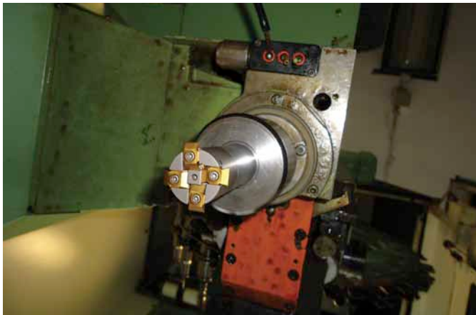
► CUTTING TOOL: GIGANT Thread Milling Cutter given by Emuge to Sharp Engineers which led to the operating time being reduced from 12 to 4.5 hrs 48
