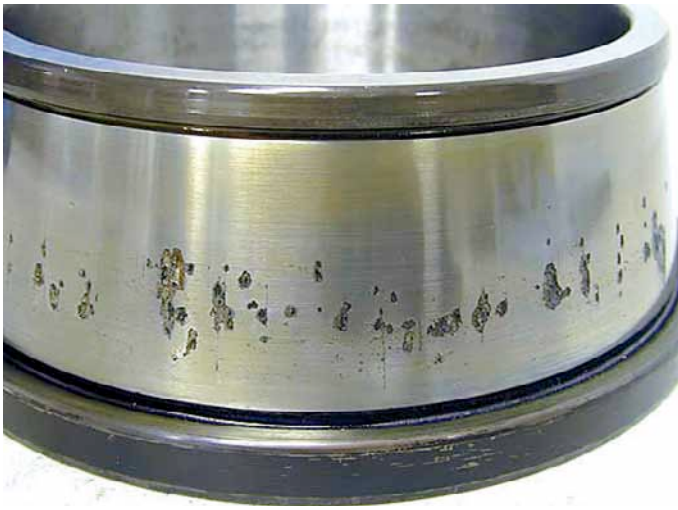
Cracks or spalls seen in wind gearboxes
