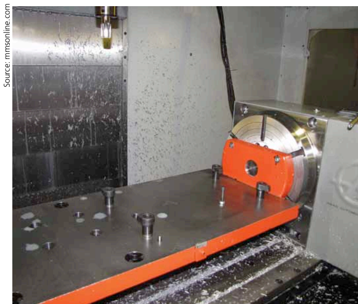
According to Indelac, the bolt-on trunnion tables were installed on the fourth axis of its Haas VF4 vertical machining center in just minutes
