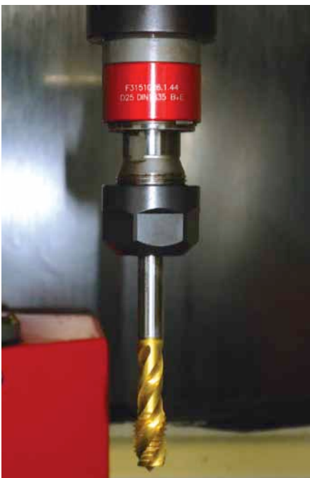
Tap holders provided by Emuge to Bosch Chassis Systems led to an improvement of more than 15 per cent and eliminated problems such as thread damage and leakage
