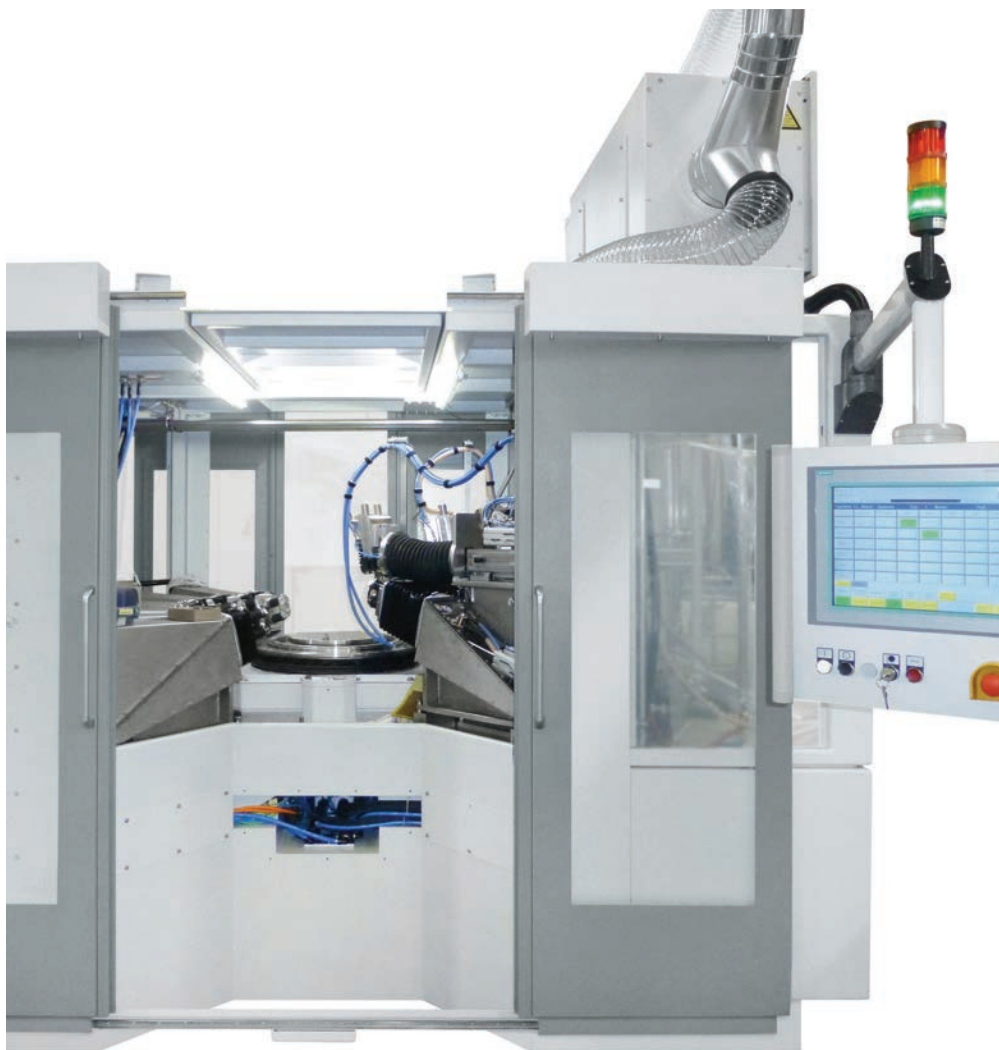
► AEROSPACE MACHINING: ECM machine with multi-stations for the machining of turbine disks in aero engine manufacture...
