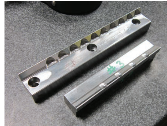
These upper and lower cutoff blades for progressive die machines exemplify the sort of short-run work that is ideal for the Trak LPMs. Although the company produces more than 1,000 of these components every year, mounting hole locations, clearances for the curved cut-outs, overall length and other attributes often vary from part to part.
