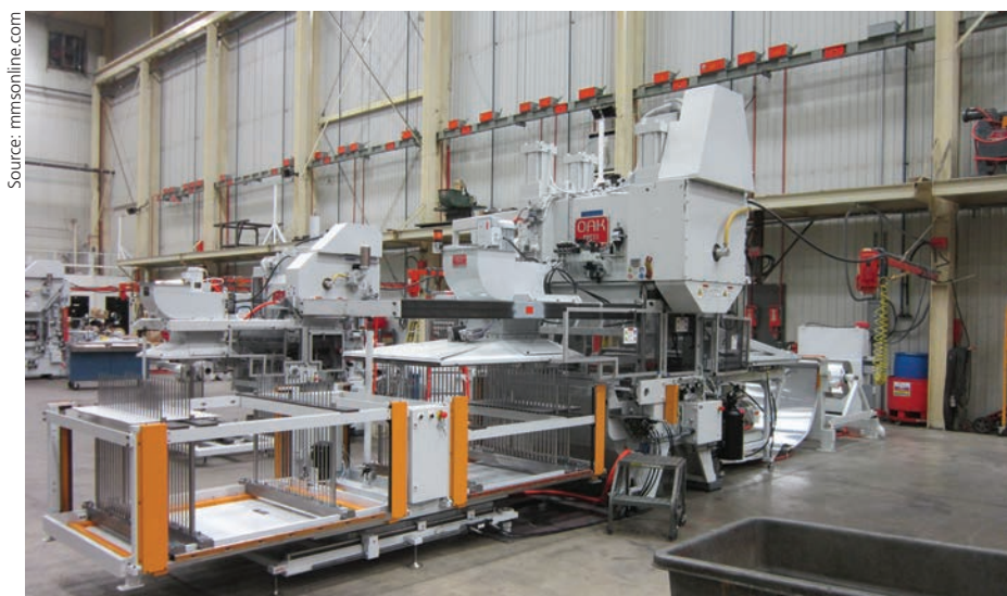
Burr Oak Tool makes equipment used in the production of HVAC systems. The progressive die press shown here is an example.
