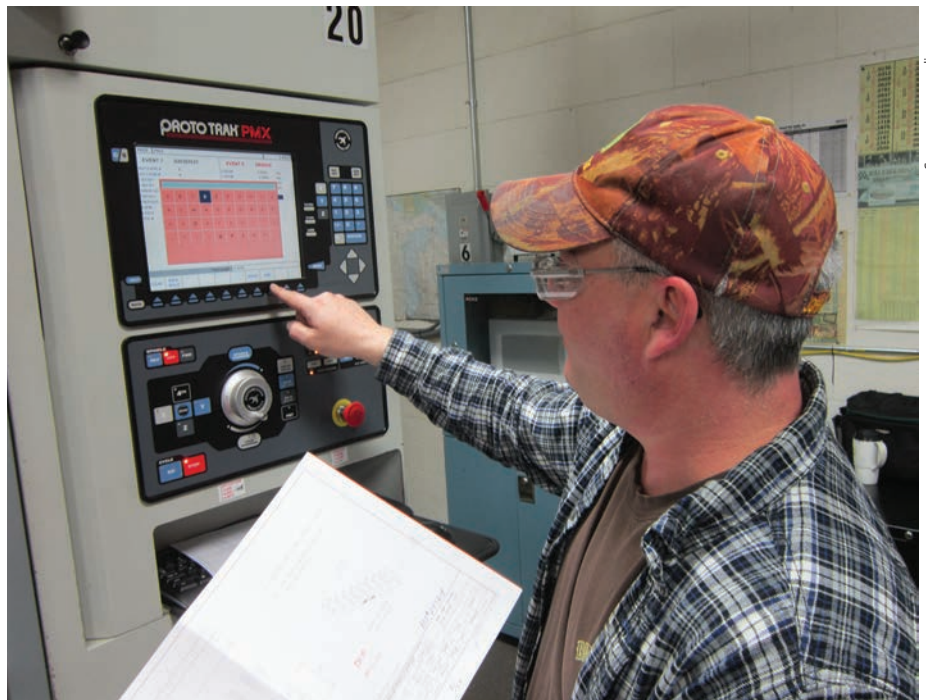
LPM lead man, John Delarye, programs a job using a conversational CNC. He attributes many of the company's gains in short-run production to control capabilities that streamline setup and change-over.
