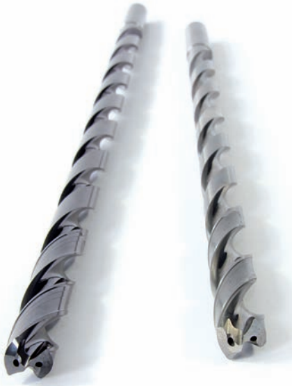
(LtoR): The deep-hole borer MEGA-Deep-Drill with special TiAlN coating is suitable for processing steel and castings while the uncoated deep-hole borer MEGA-Alu-Deep-Drill is suitable for processing aluminum and non-ferrous metals
