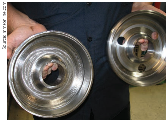
FIG 2: This round part is an obvious candidate for turning, but in fact turning is now used only for finishing cuts. High-speed milling on a machining center has proven to be a more effective way to rough out the stock.
