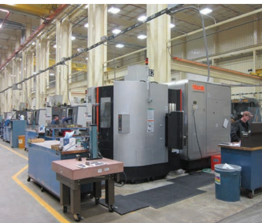
These HMCs handle most of Burr Oak's higher-volume work. Operators inspect parts at the machines using height and surface gages at each station.
