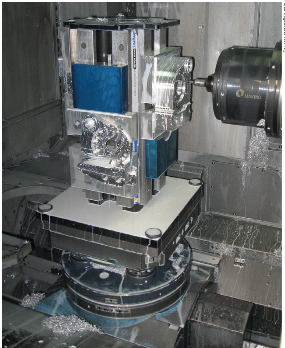
FIG 1: The freedom to machine various surfaces of a part in one setup accounts for part of an HMC's efficiency advantage, but Advance CNC Machining says the benefits extend well beyond this.
