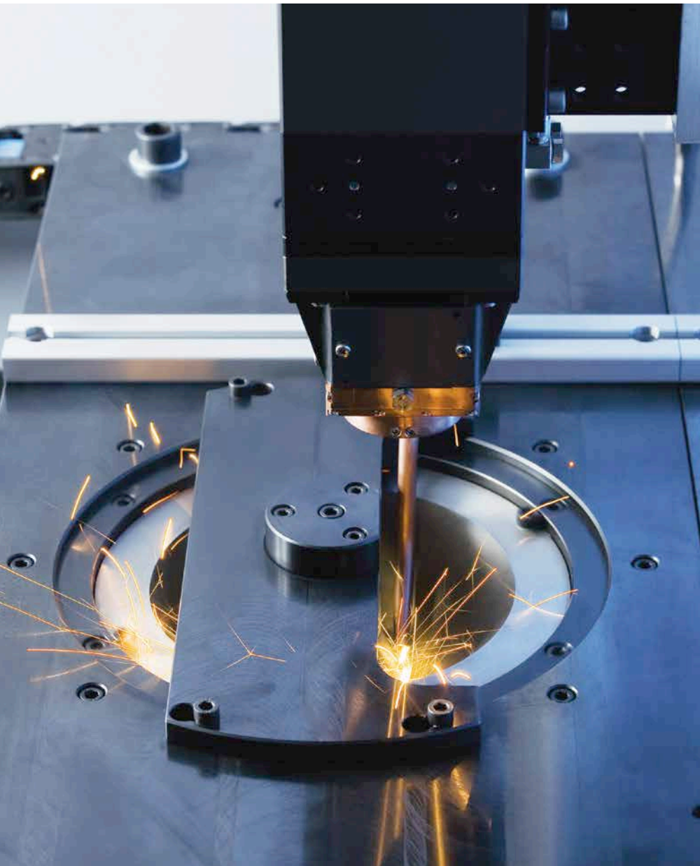
Laser welding a synchronous wheel onto a gear
