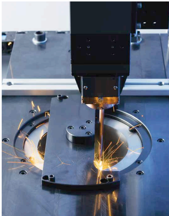
► LASER WELDING: Laser welding a synchronous wheel onto a gear
