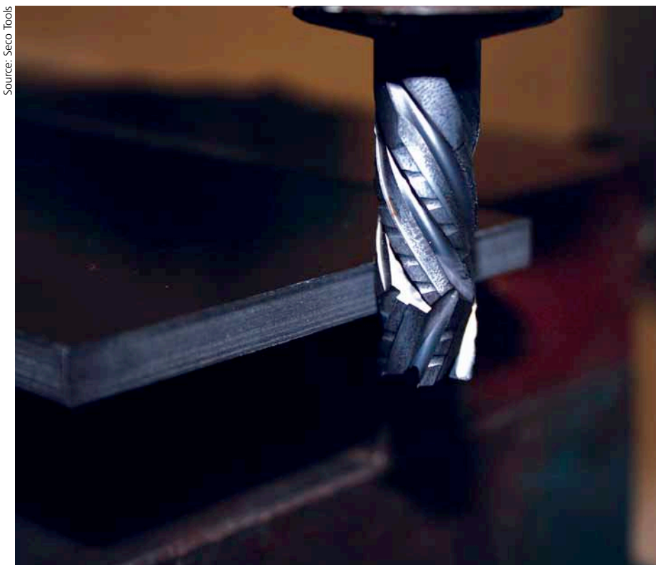
Double helix rougher with chipbreakers
