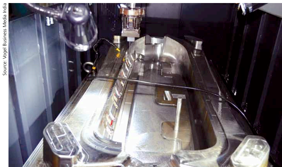
Mold being manufactured at Sridevi, using CAD/CAM integration, which ensures an error-free and highly accurate process
