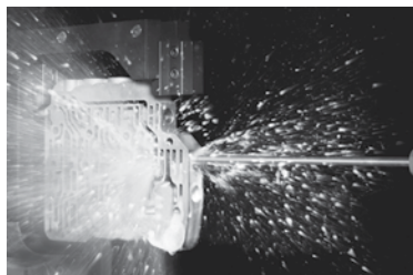
Simultaneous de-burring, chip removal and cleaning of workpiece using high pressure water jet with pressure of up to 2,000 bars
