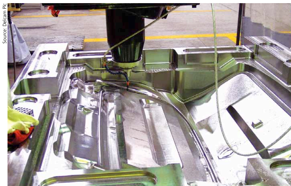
Large tool milled using PowerMILL 5 Axis
