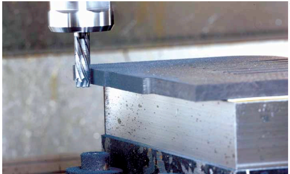
Multi-flute tool with chip breakers for roughing operations
