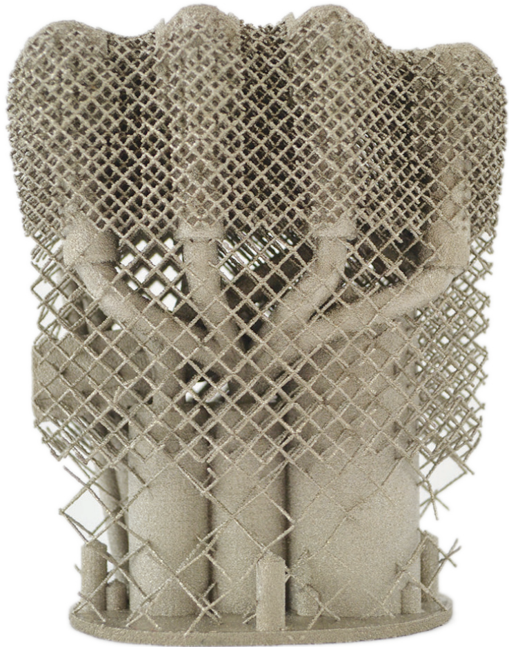
► ADDITIVE MANUFACTURING: This component of a humanlike robotic hand illustrates various features of a part designed for additive manufacturing. 42
