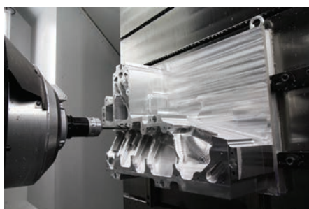
► EVENT REPORT: A view of the roughing of the component to be used in the Bloodhound SuperSonic Car.
