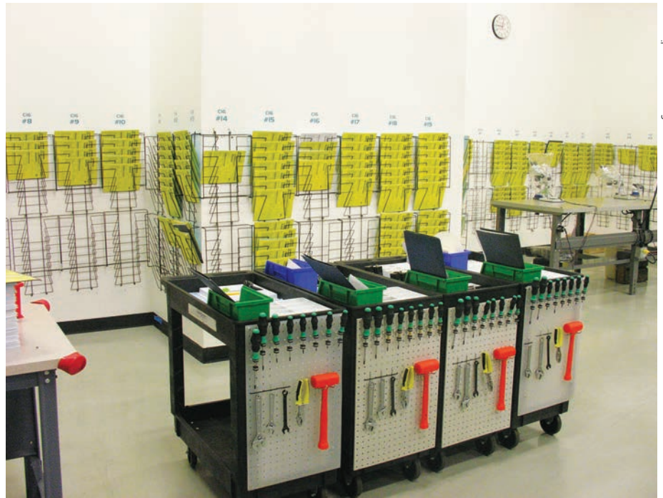
FIGURE 1: The shop prepares job carts like these to streamline setups. These carts contain cutting tools, hand tools, gages, instructions and virtually everything else required to set up a machine for a new job.
