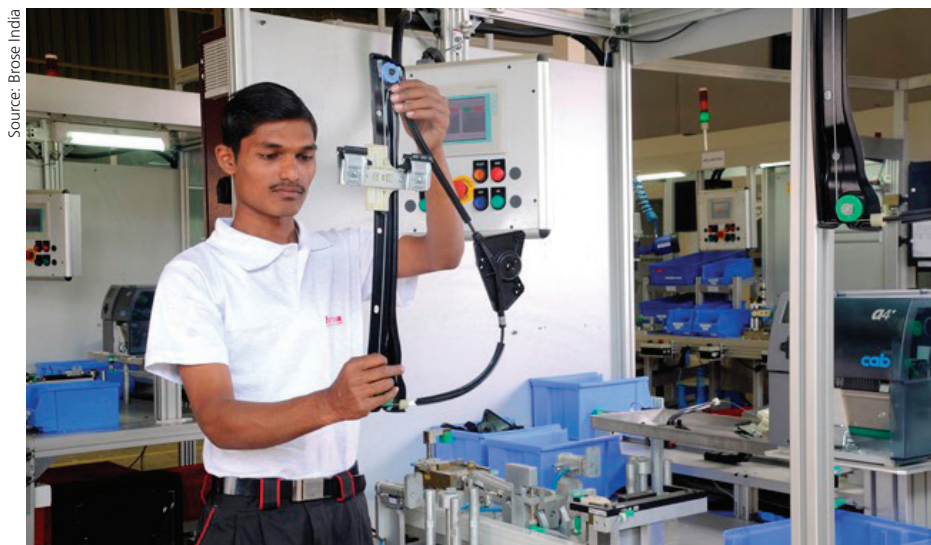
Window regulator being assembled in the Brose's new facility in Pune.
