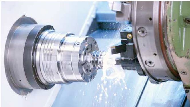
► WORKHOLDING: Going from OD to ID to three-jaw chucks is accomplished in a matter of minutes
