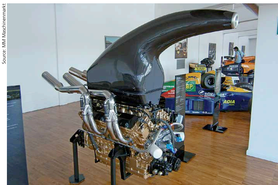
A CFRP intake manifold on a Lamborghini engine for a racing boat
