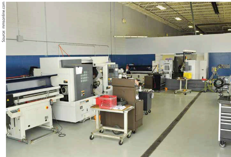
All of the turning centers on RFM's shop floor are bar fed. A low-volume and high-mix production has driven the company to look for quick-change options in its workholding.
