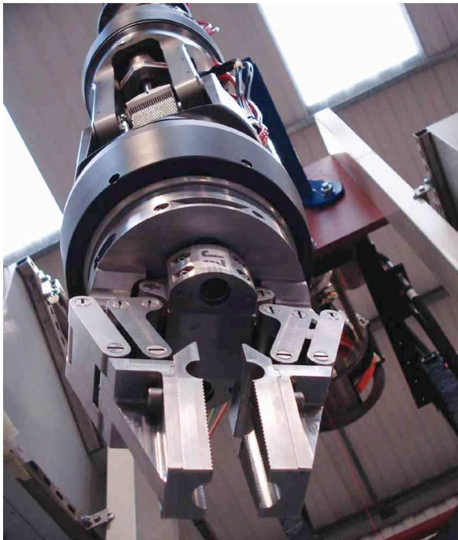
► NUCLEAR ENGINEERING: With the help of solutions from National Instruments, James Fisher Nuclear Ltd could develop manipulator for decommissioning nuclear plants
