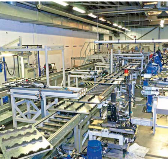
► MATERIAL HANDLING: Material carriers run through the assembly plant at Thomas Regout
