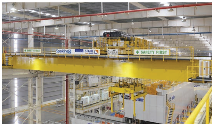
► MATERIAL HANDLING: The heart of the crane systems are SHW8 rope winches from STAHL CraneSystems. During production in Künzelsau they were equipped for particularly high speeds and operating with tool grabs. 54
