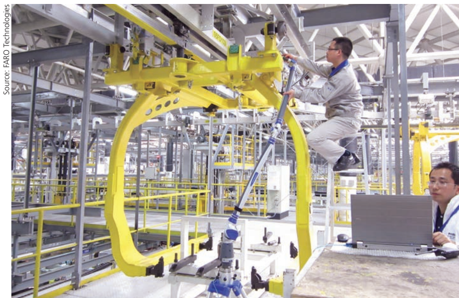
The FaroArm is used for alignment checks on the center axis of the conveyor trolley.
