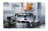
be clamped gently and without warping and be machined on five sides in a single operation. If MAGNOS square pole plates are equipped with an interface on their base side to the VERO-S quick-change pallet system, they can be changed on the machine table in just a few steps.
