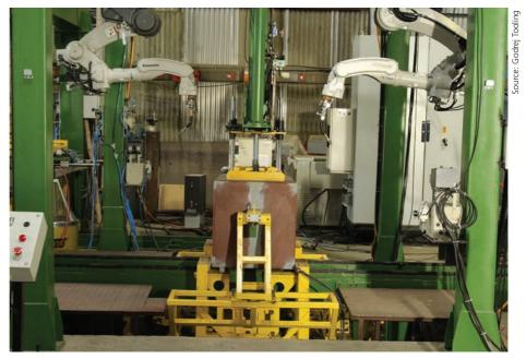
Inverted welding robot being used at the facility.
