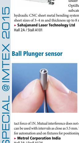
The Ball Plunger sensor by Metrol Corporation India is one of the world's smallest sensors housed in a compact design starting with diameter 4x12 mm length and M5x19 mm length. The contact can be of straight, sliding, angled touch types. The sensor comes with a minimum required con-
