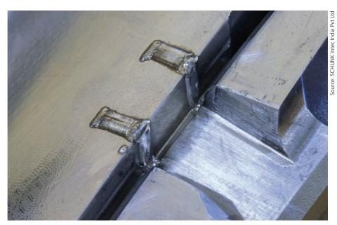
Partial energy transfer and special pulse shaping prevent stress and cracks from forming in tools during repair welding.
