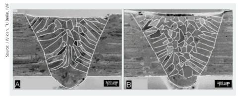
Pulse modulation can be used to achieve a homogeneous structural distribution, as shown here in Al 99.9.
