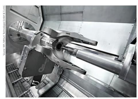
Heavy duty cutting places particular requirements on the machine and working processes. A material such as titanium is hard to cut and specific know-how is necessary to deal with these requirements.
