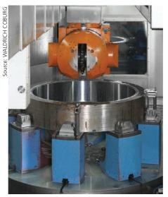
The clamping device is an innovative in-house development from Siemens AG.
