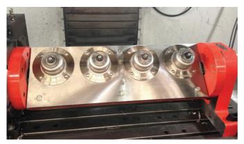
► VERTICAL MACHINING CENTER: The trunnion table enables Vertiflo Pump to machine as many as four parts at a time, cutting per-part cycle times in half.
