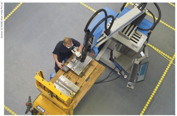
Laser welding in threedimensional space demands flexible machinery.
