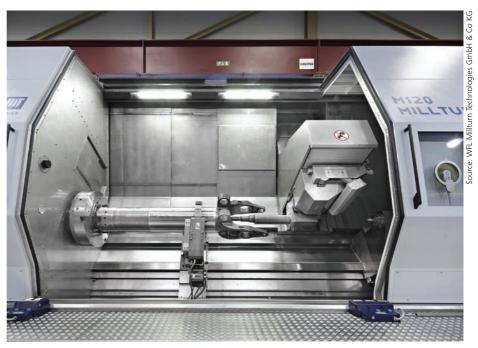
The WFL M120 Millturn machine has been developed for machining hard to cut materials such as titanium
