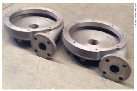
Pump parts that require milling and drilling at 90° can now be machined in a single setup instead of two.
