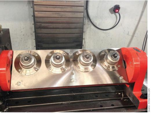
The trunnion table enables Vertiflo Pump to machine as many as four parts at a time, cutting per-part cycle times in half.
