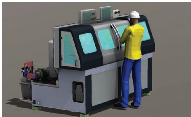
► MANUFACTURING SOFTWARE: Gun drilling machine design using SolidWorks software
