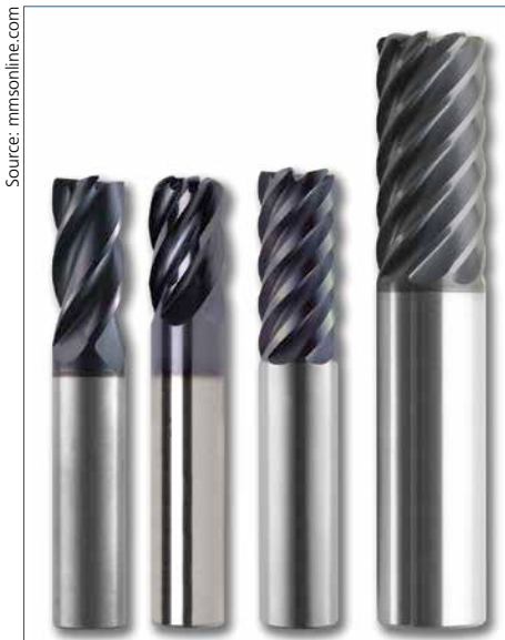
The three smaller end mills shown above have four, five and six flutes. When programming a cutter for an operation that requires more engagement between the cutter and workpiece (as in traditional roughing), choose the smaller number of flutes.
