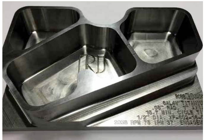
► MACHINING: Machining this titanium workpiece, which could fit inside a cigar box, is a manageable job for today's generation of machining centers
