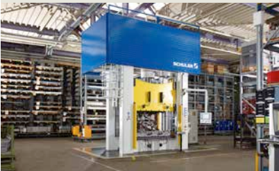
Two hydraulic 400-ton systems from the HPX series are in operation at König Metall's stamping and press plant in Croatia.
