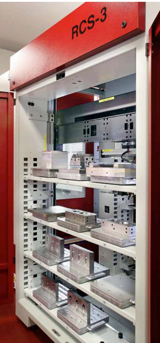
The 38-position pallet change system that feeds the Roeders RXP601 DSH.
