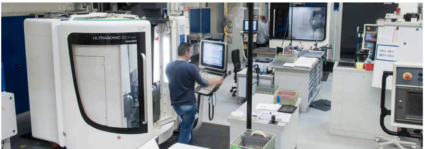
► ULTRASONIC TECHNOLOGY: While CeramTec machines numerous workpieces with conventional grinding machines, the ceramic experts now also have three 5-axis ULTRASONIC machines at their disposal.
