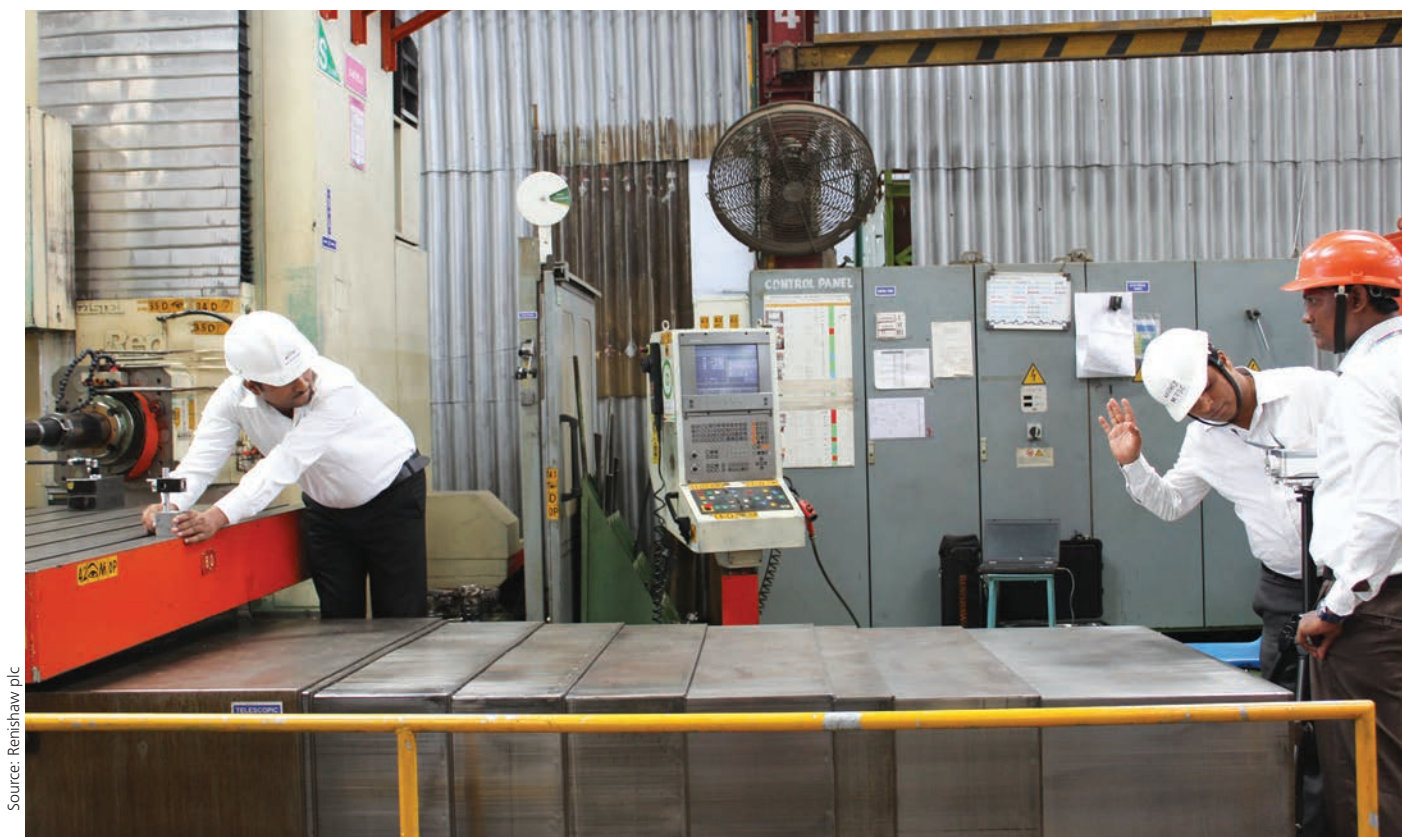
Godrej personnel calibrating a CNC machine with an XL-80 laser.
