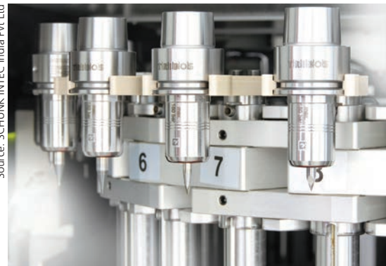
The SCHUNK TRIBOS RM precision toolholder is also available in an ultrafine balanced version with a balancing grade of G 0.3 at 60,000 rpm.
