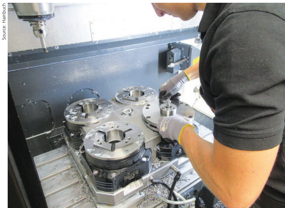
In the hydraulic stationary chucks there is no longer any room for chips, and changing from O.D. clamping to I.D. clamping is quickly accomplished.
