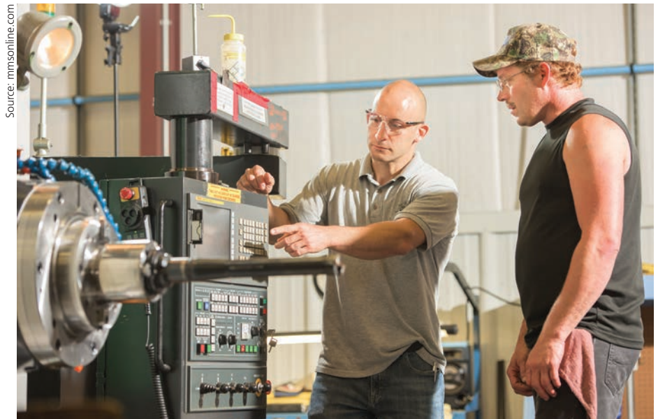
Machinists Dale Penkaty and Troy Dorman operate the Doosan Infracore DBC 130 horizontal boring machine where the closure head was machined. With Sandvik's tooling, the men could complete a part in a single shift, a 90 per cent time savings compared to the previous process.
