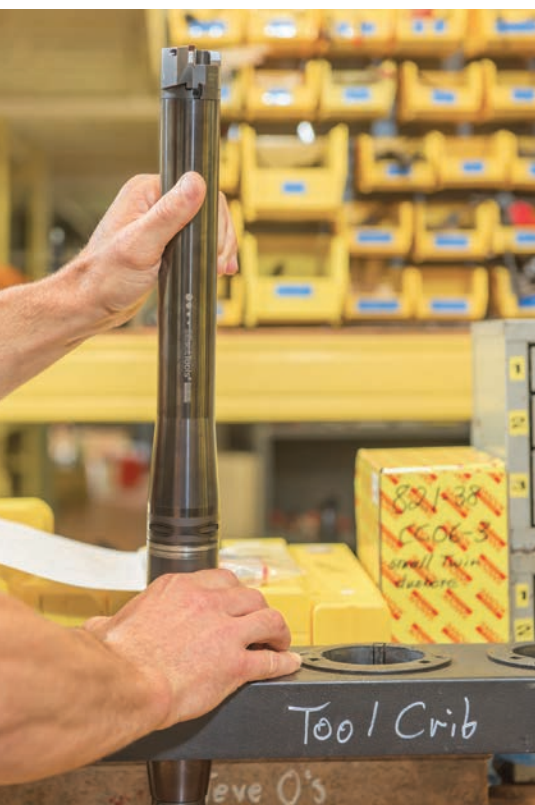
The boring tool sticks out around 11 inches from the spindle face, so reducing vibration during the boring process was critical.
