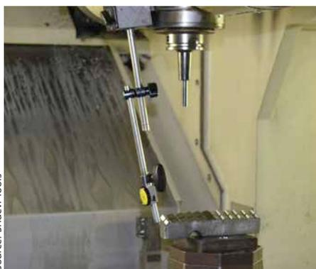
Inspection being conducted on the contoured shape of completed job at Sridevi Tools
