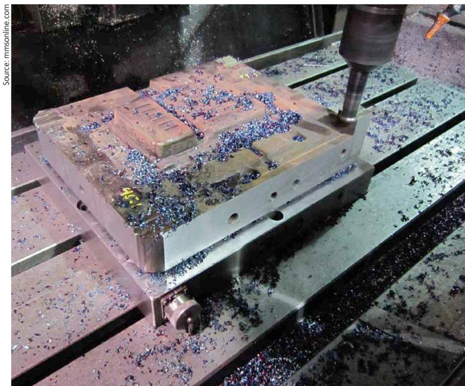
Electropermanent magnetic chucks on the company's sinker EDMs and machining centers speed setups and enable multiple jobs to be fixtured at once
