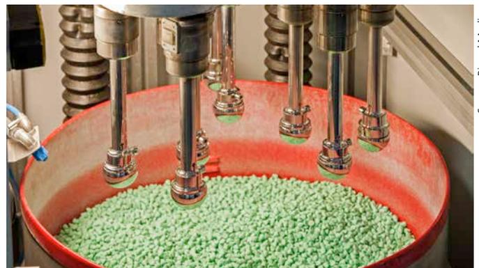
Cast or forged implants go through processes like three-stage OTEC dry polishing
