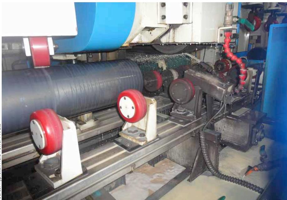
The job passing to the multihead belt grinding machine at the Hypratek facility
