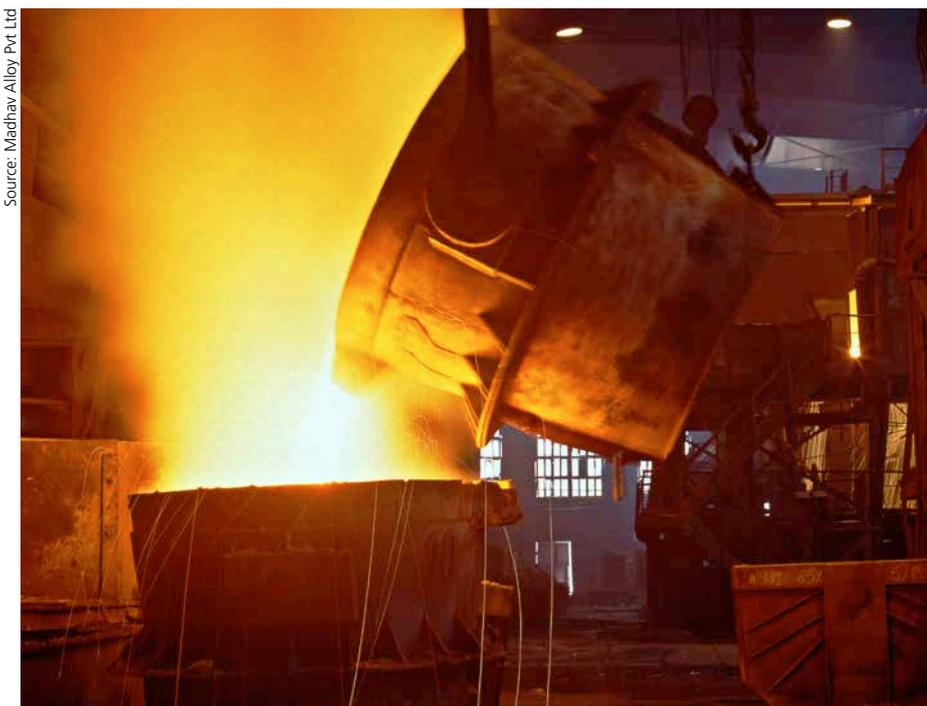
Typical casting of molten iron at a steel plant
