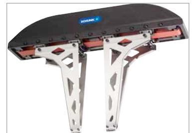
The CGH long-stroke gripper from SCHUNK is the result of modern simulation methods, intensive test series, and economic manufacturing processes. This lightweight and rigid gripper has a correspondingly torsional stiffness. At a weight of 11.7 kg, the CGH disposes of a gripping force of 2,500 N and a variable stroke per gripper finger of up to 160 mm. The decoupled re-circulating ball carriages ensure that the acting moments will be optimally distributed onto the whole rolling elements.
