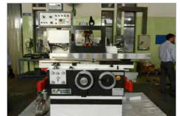
reliability increases with its ease of operation, desired sub-micron level roundness and size accuracies. Wheel slide of the machine moves on precision linear bearing guideways ensuring repeatability within  $\pm 0.001$  mm. Moreover, this machine is designed and manufactured to meet higher end European EC standards for safety and environment.
