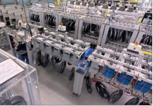
reliability – only those who conduct intensive research and testing will successfully bridge this gap. The industry's largest test lab conducts more than two billion test cycles per year on a total of 107 test rigs.
