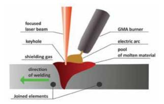
acting as a support to the weld pool make the welding process faster and smoother with minimal adjacent heated area. So for the applications that would require ten passes on weld tube, can be done with maximum of one pass or two pass welding.
