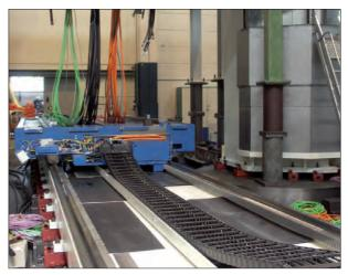
Holding chainflex<sup>®</sup>-cables in e-chains<sup>®</sup> for motion-control applications.
