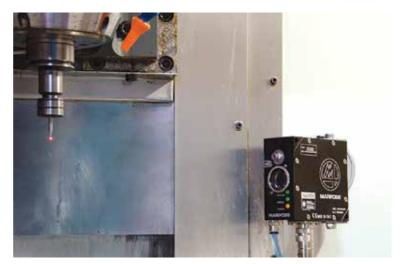
Fast and reliable detection achievable by the TBD allows to reduce production time and to avoid expensive work-pieces scrap due to wrong cutting process by damaged or broken tools.
