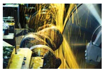
JUCRANK pendulum grinding machines take care of almost every conceivable crankshaft grinding operation.
