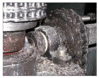
Dry-running igubal<sup>®</sup> plastic spherical bearings – no chip adhesion.
