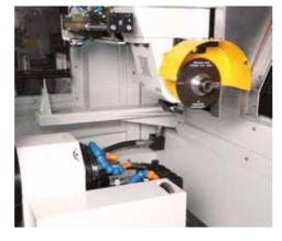
which enables regular interval of Dressing for grinding wheels and also different radius in the wheels can be dressed by programming. This enables in reducing cycle time in manufacturing taps with higher flute finish. Simple arm type automation is also provided for pick and place operation. This in turn reduces operator intervention and reduces man power for mass production line. As automation is configured within machine axes, overall cost of automation is also not very much expensive
