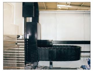
igus<sup>®</sup> E2 e-tubes, upright and rotated by 90° in the chip area.
