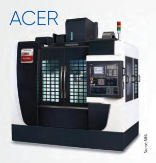
Acer, the high-performance Vertical Machining Centre from Ace Micromatic Systems, promises high accuracy and enhanced productivity. The machine has a rigid structure and ergonomic design, and is loaded with a high-speed spindle, high-precision roller guideways and ball screws. A wide door opening fixture allows the components to be easily loaded and unloaded from the machine.
