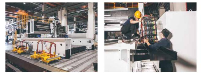
In its robotic machining centres, many companies use fully harnessed energy chain systems from igus. This cuts out many process steps for the manufacturer, reducing assembly time from several weeks to just half a day. Another benefit receives is from a single source and delivered onsite fully-tested for reliability and safety.
